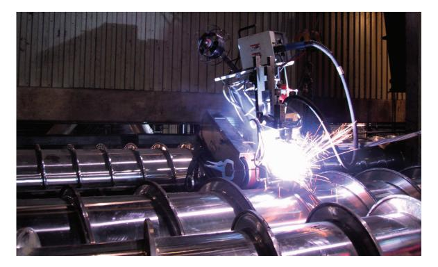
Twin screw presses in operation are subject to wear and abrasion. The clearance between the top of the screw flights and the strainer plates has an influence on the press performance. This is the area which is most exposed to wear and abrasion. Consequently, after a certain time the performance will be reduced and the flights should be rewelded to regain their original diameter.
